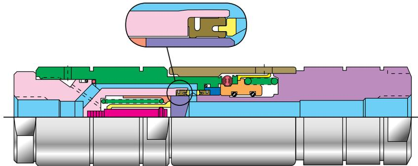
The balanced design is Snap-tite's latest design improvement for sub-sea application. The separation force is typically less than 100 pounds (45kg) for each coupling while pressurized internally to 10000 psig (690 bar). Spillage and water ingress are nearly eliminated and the envelope is only slightly larger than that of most commonly used poppet couplings.
