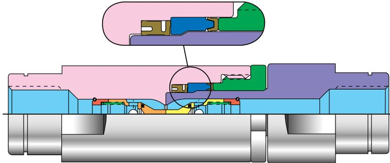
The poppet design coupling is the most commonly used for sub-sea applications. The simple proven design is reliable and economical.
