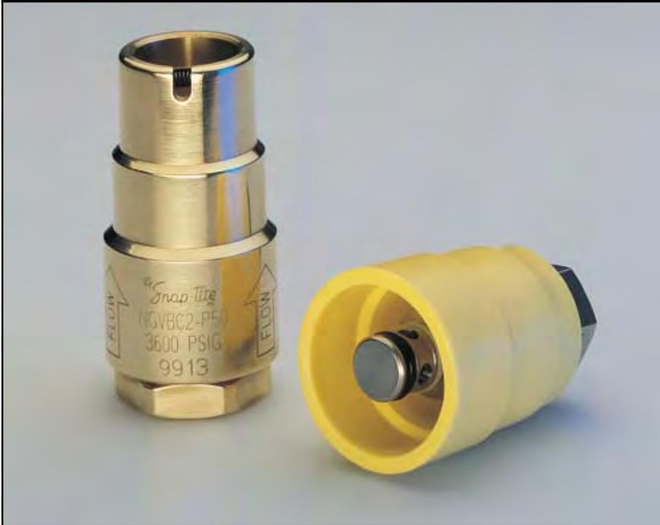
Snap-tite's inline breakaway is designed specifically for compressed natural gas fueling systems. When properly installed, this inline breakaway allows for the safe disconnection from the fueling system without damage to the dispenser in the event of an accidental disconnect (drive-off). The inline breakaway was designed to replace the traditional tripod leverage towers used in conjunction with the ISO B style coupling as the breakaway connection for the fueling hose from the dispenser.
