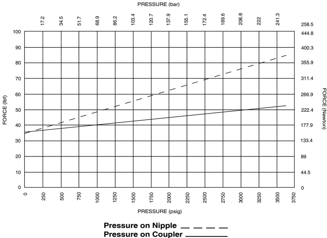
**NOTE:** By comparison, it would take approximately 40 lbs (177.9 Newton) of force to connect a standard 1/2" ISO 16028 coupling with 200 psi (14 bar) internal pressure.
